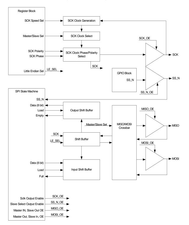
Figure 13. SPI Block Diagram
